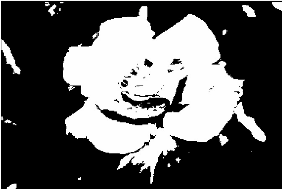
Figure 4.14: To implement Thresholding of image using mean as a threshold value and half of the maximum pixel value of image
