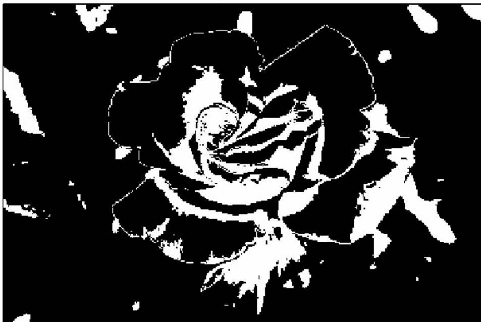
Figure 4.38: To implement Bit Plane slicing of gray scale image
