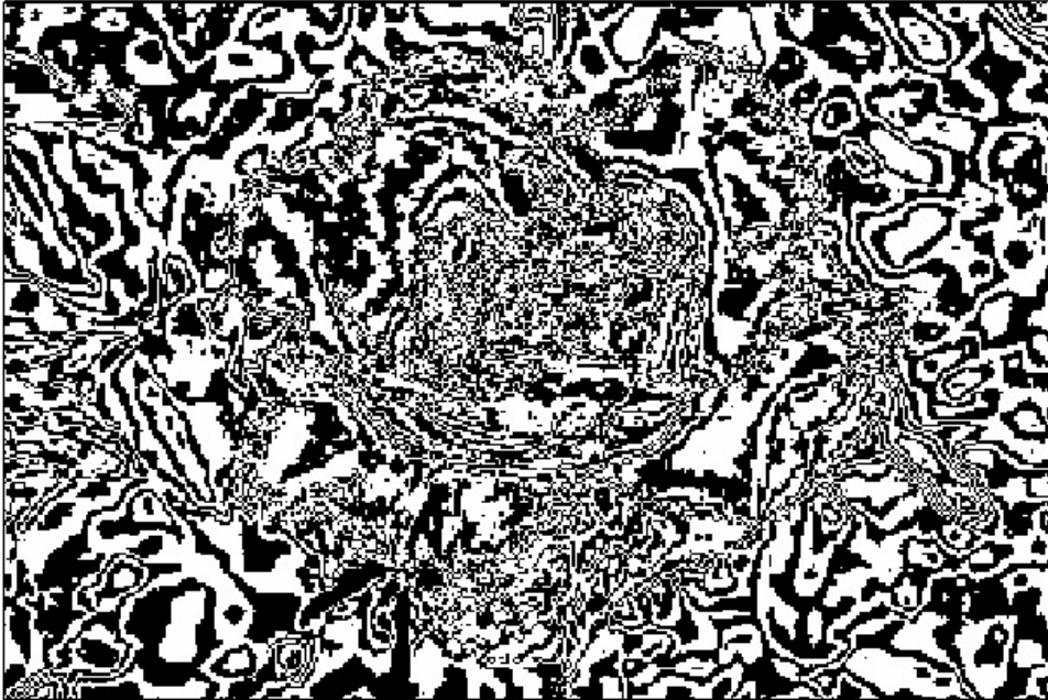
Figure 4.35: To implement Bit Plane slicing of gray scale image
