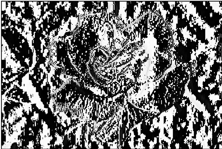
Figure 7.10: To Implement Image segmentation discontinuities using edge detection Robert Operator
