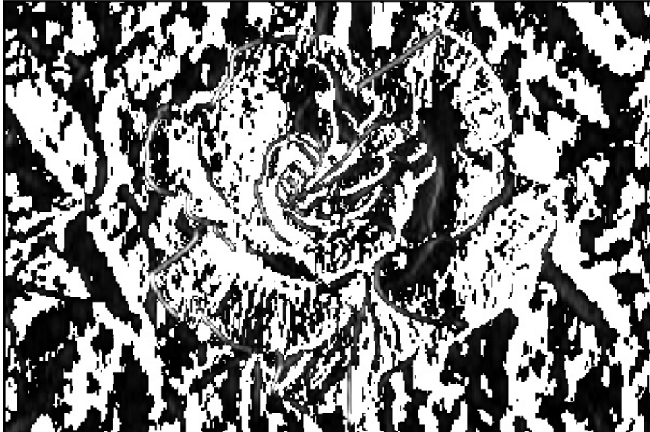
Figure 7.13: To Implement Image segmentation discontinuities using edge detection prewitt operator
