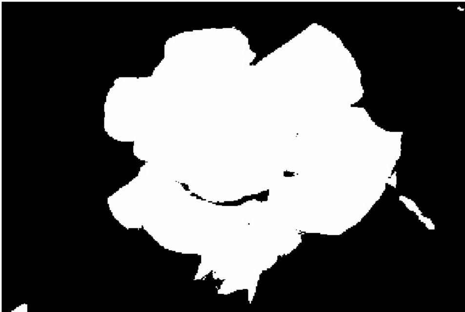
Figure 4.19: To implement Thresholding of image using mean as a threshold value and half of the maximum pixel value of image
