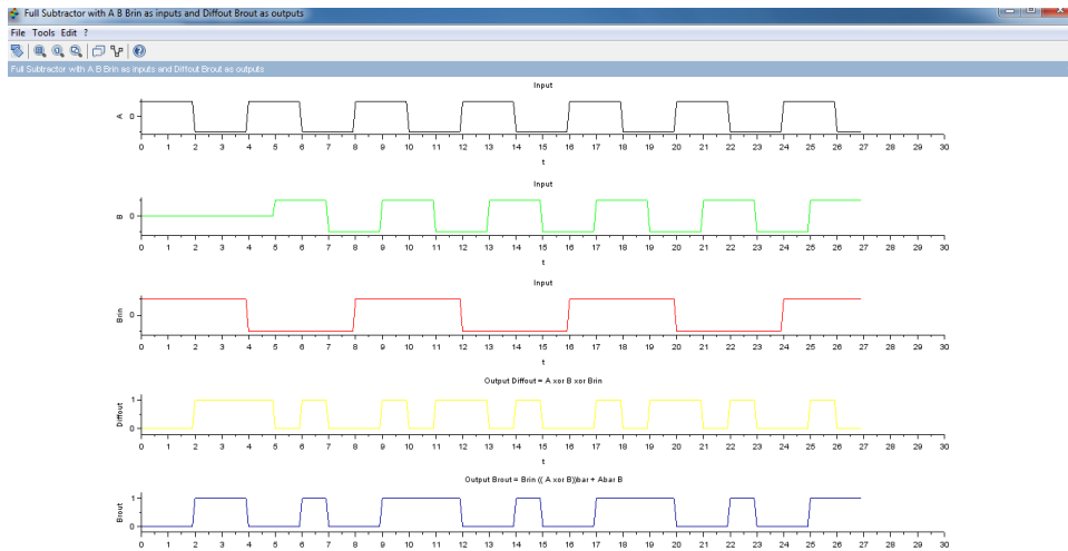
Figure 3.4: Full Subtractor Design
